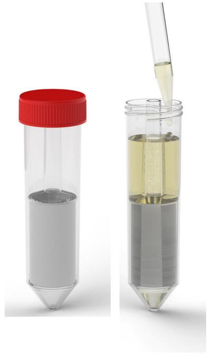
Remove the red Lid from the 15 ml (S) / 50 ml (L) Tube and open device.
