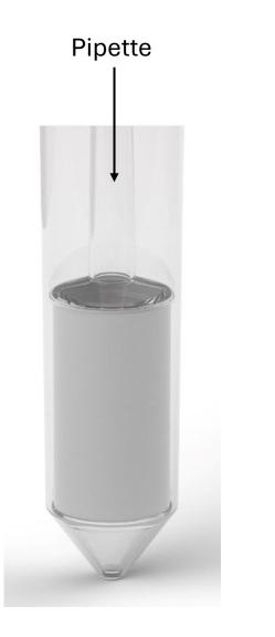
If the filtration has not reached the final required end point please remove the filtrate from the inner part of the device by placing a pipette down the center of the device.
