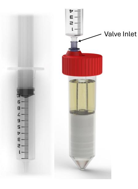
Pull back the plunger of the 10 ml syringe and then push the syringe into the Pressure Cap valve inlet.
